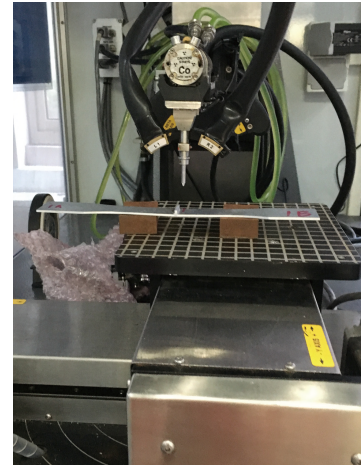
图2 残余应力测试 Fig.2 Residual stress test
